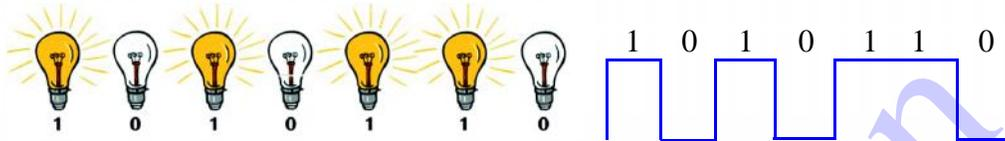
Fig. 1.8 : Digital representation of ON and OFF states
