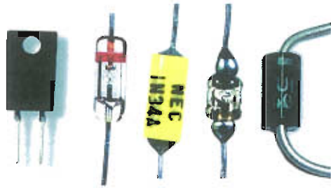
Fig. 10.5 Different types of diodes
