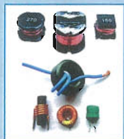
Fig. 10.2 Different types of inductors
